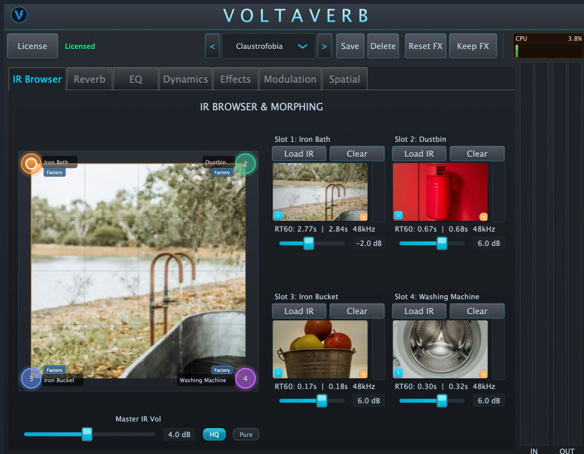
The IR Browser with four impulse responses loaded and the XY morph pad
