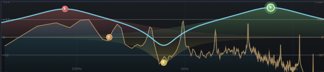
Real-time spectrum analyzer with EQ curve overlay and draggable band nodes
